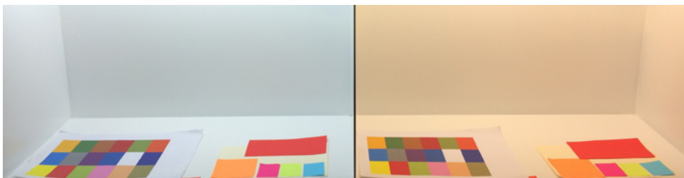
Figure 9. Examples of colour temperatures. A colour temperature of 4 000 K is shown on the left, and of 2 700 K on the right.
