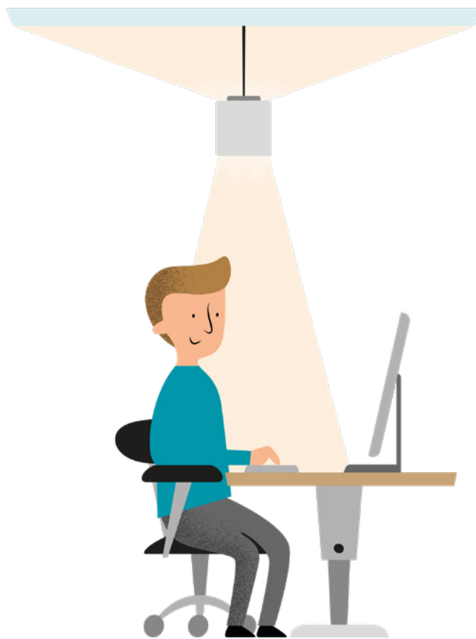
Figure 7. Principles for luminaires placement. The luminaire must be positioned above and parallel to the front edge of the desk. A suspended luminaire with both indirect light (from the ceiling) and direct lighting often provides a good luminance distribution.
