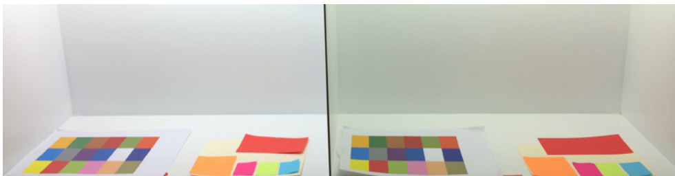
Figure 8. Examples of colour rendering. R_a index of 90 on the left, and of 80 on the right.
